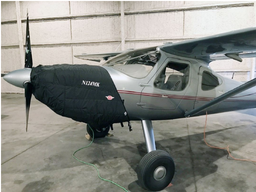
Glasair Aviation Glastar, Sportsman 2+2 Insulated Engine Cover
