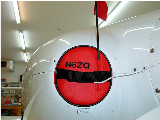
Lancair 320 Engine Inlet Plugs
