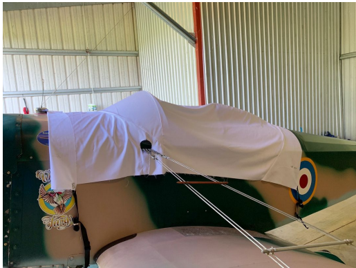
Bowers Flybaby Canopy Cover, test fit design
