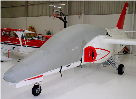
S-211 Canopy/Nose Cover & Engine Plugs
