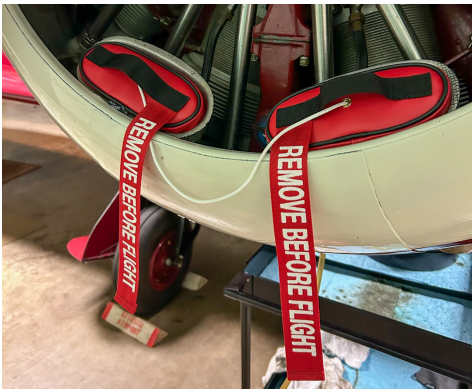
Beech Staggerwing Carb Inlet Plugs, Located Inside Engine
