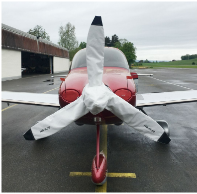
Cirrus SR22 Propellor/Spinner Cover and Inlet Plugs
