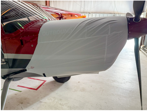
Rans S-21 Engine Cover, test fit cover
