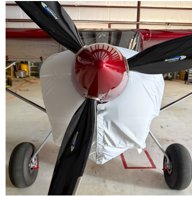
Rans S-21 Engine Cover, test fit cover
