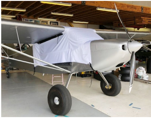
Rans S-20 Canopy Cover, test fit cover
