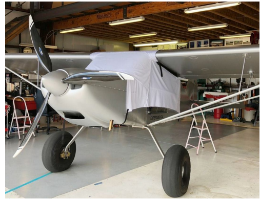
Rans S-20 Canopy Cover, test fit cover
