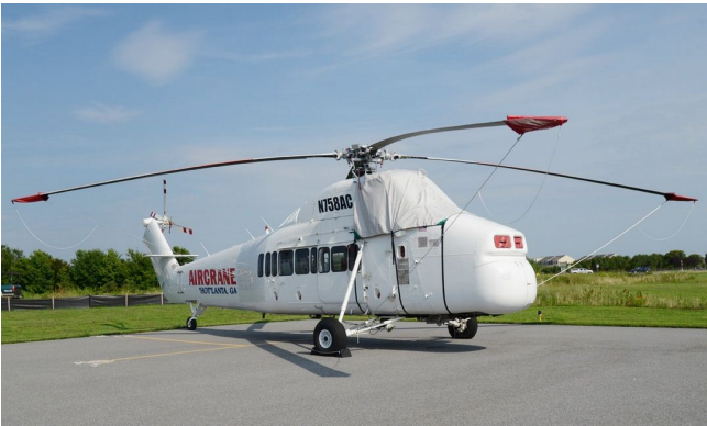
Sikorsky S58T Rotor Hub, Tail Rotor Hub, Engine Plugs, Blade Tie-Downs Sikorsky S58T Cockpit Cover, Intake Plugs, Blade Tie-Downs
