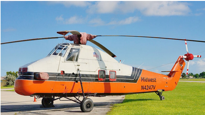
Sikorsky S58T Rotor Hub, Tail Rotor Hub, Engine Plugs, Blade Tie-Downs Sikorsky S58T Cockpit Cover, Intake Plugs, Blade Tie-Downs
