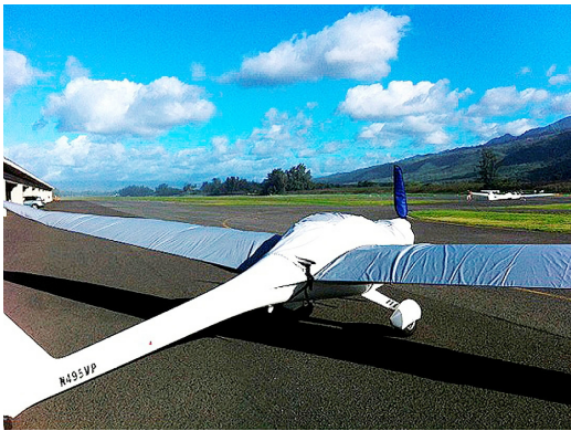
Lambda Canopy/Engine Cover and Wing Covers
