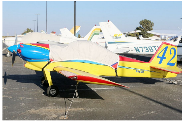
Van's RV-3 Canopy Cover and Engine Plugs
