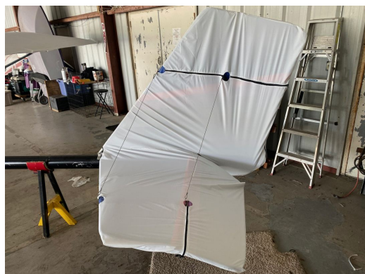
Rans S-12 Empennage Cover, test fit
