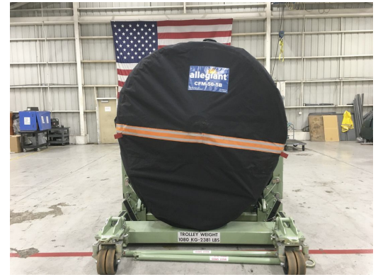
CFM56-5B Off Link Cover, fully enclosed
