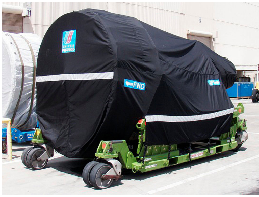
PW 2000 SERIES OFF-LINK ENGINE COVER, "rain cap" style
