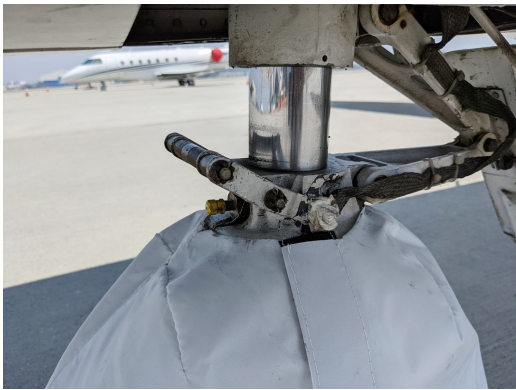
CJ1 Nose Gear Tire Cover, test fit
