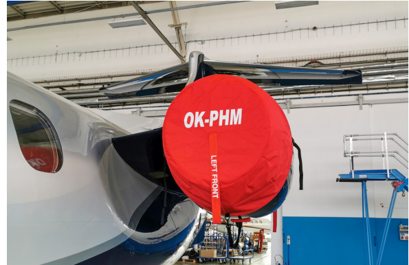
Embraer Phenom 300 ENGINE INLET COVERS & EXHAUST PLUGS (includes lower nacelle plug) (set of 6)
