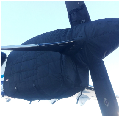
ATR-72-202 Insulated Engine & Prop Hub Covers
