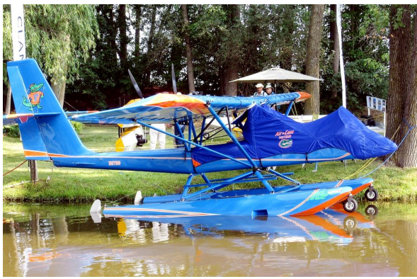
CANOPY/NOSE/BAGGAGE AREA COVER, with aft flat windshield
