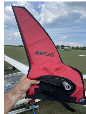
Schempp-Hirth Ventus-2B winglet/wingtip pads
