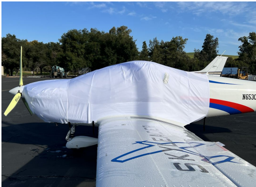
Jihlavan JA-600 Skylander Extended Canopy/Engine Cover, test fit cover
