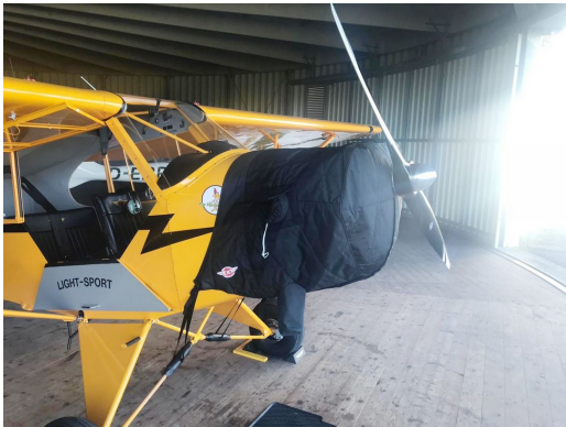
Legend Cub AL3 Insulated Engine Cover with special preheater access vent and attachment detail and fully enclosed under cowling. Piper J3 Cub Travel Weight Canopy & Engine Cover
