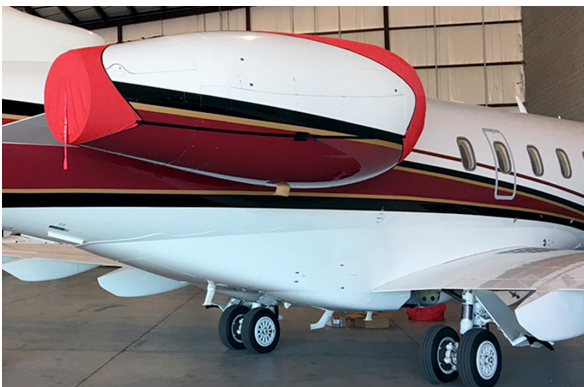
Intake/Exhaust Covers, 3-Strap Type. Successfully installed by two crew, one stepladder.
