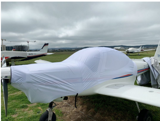
Grob 115 Canopy/Engine Cover, test fit cover
