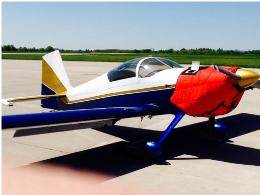
Van's RV-7 Insulated Engine Cover
