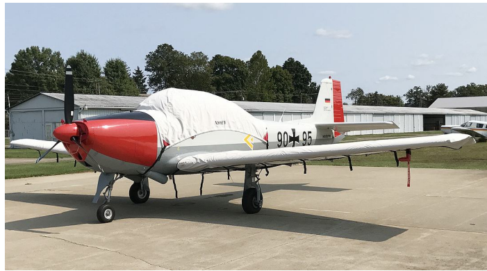
Focke Wulf F149 Canopy Cover, Wing Covers, Engine Plugs ENGINE PLUGS PREVENT BIRD NEST FOD. Piper Saratoga Engine Cowling Bird's Nest
