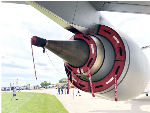
McDonnell Douglas DC-8 Exhaust Plugs, Donut Ring Type For Bypass Vent And Exhaust McDonnell Douglas DC-8 Exhaust Plugs
