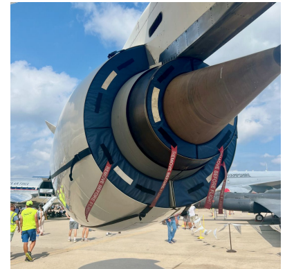
McDonnell Douglas DC-8 Exhaust Plugs, Donut Ring Type For Bypass Vent And Exhaust McDonnell Douglas DC-8 Exhaust Plugs
