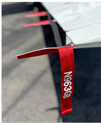
Cessna Citationjet 525C, CJ-4 Static Wick Protectors, 3 Per Wing, 1 On Tailcone Area
