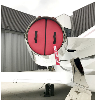
Cessna Citation 680 Exhaust Plugs, folding type
