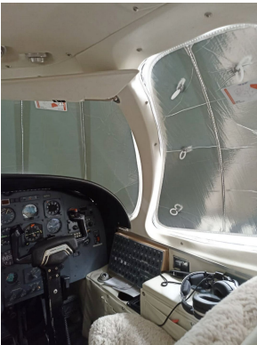
Cessna Citation I & II Cockpit HeatShields
