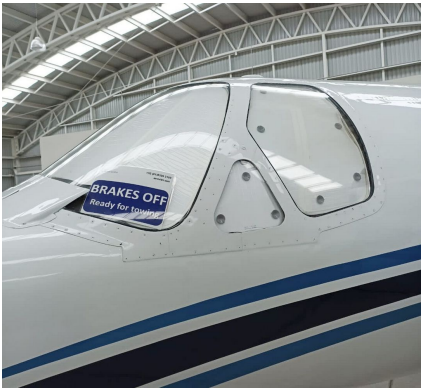
Cessna Citation I & II Cockpit HeatShields
