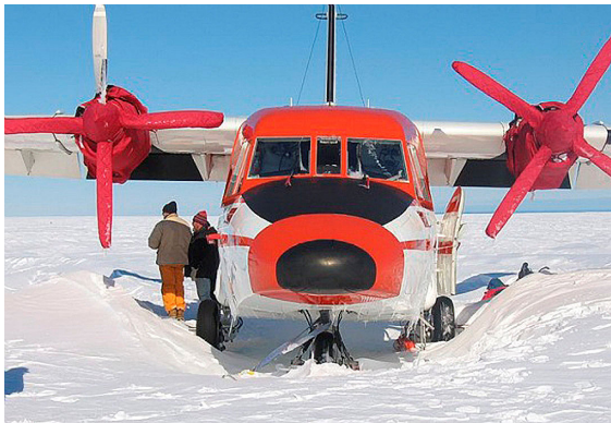
Casa 212 Insulated Engine & Propellor/Spinner Covers
