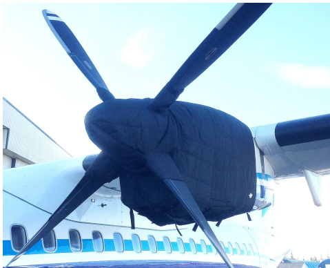
ATR-72-202 Insulated Engine & Prop Hub Covers
