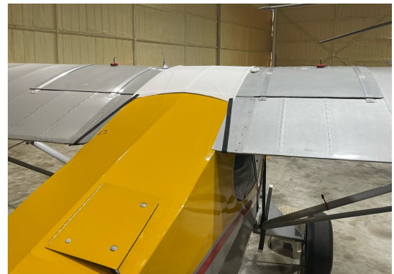
Piper J5A Windshield/Skylight Cover, test fit
