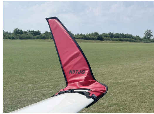
Schempp-Hirth Ventus-2B winglet/wingtip pads
