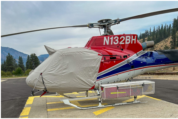
Eurocopter AS350-B3 Bubble Cover w/Wire Strike & Cargo Mirror details.
