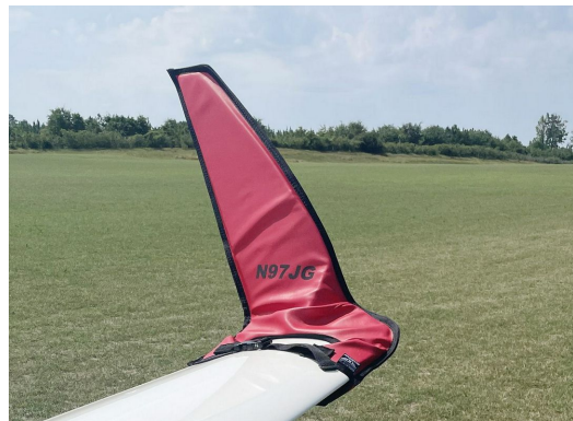
Schempp-Hirth Ventus-2B winglet/wingtip pads
