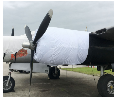
Douglas A-26 Engine Cover, test fit cover
