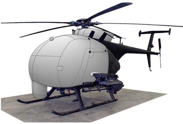
MH-6J Bubble, Flir & Doghouse Covers (illustration)
