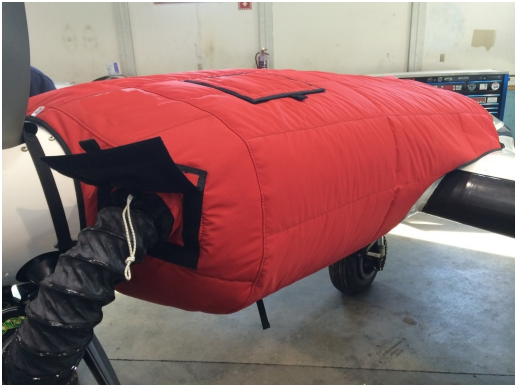
Cessna 402 Insulated Engine Cover with Heater
