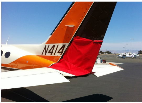
Cessna 414 Rudder Openings Cover (bird barrier)
